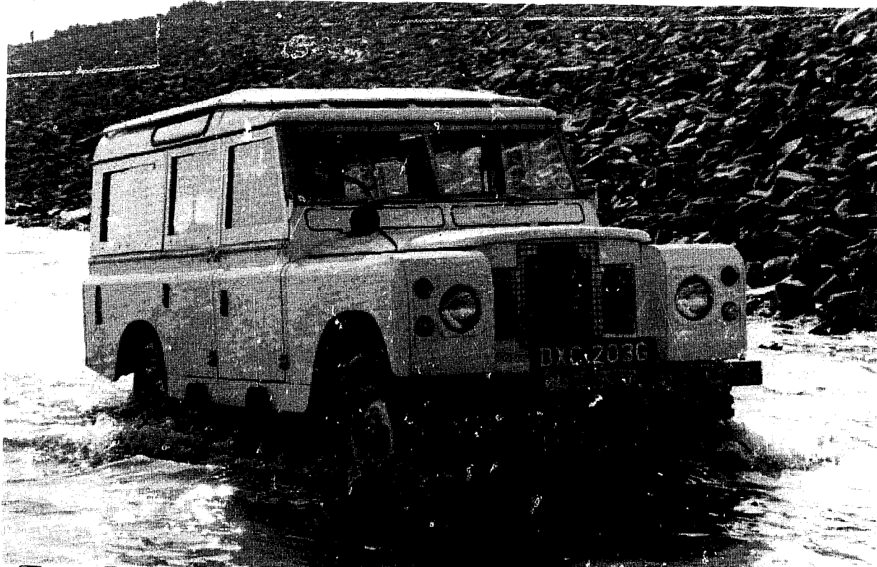
LAND ROVER has been the standard 4WD vehicle in many parts of the world over an extended number of years, resulting in widespread distribution and ready availability of parts and service. The Land Rover is available in 88 and 108 inch wheelbase chassis sizes, as well as a larger forward-control model. Bodies include pickup trucks, soft or hard top, and the station wagon body which is illustrated above on the 108 inch frame.
