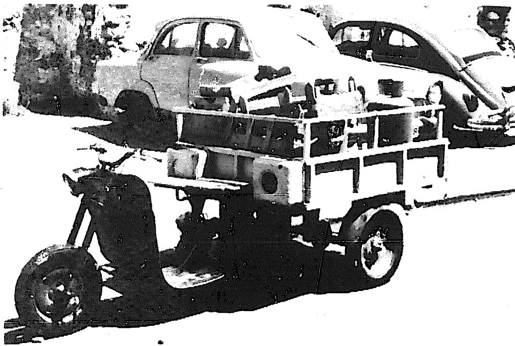
Urban goods vehicle, manufactured in Greece. 50cc engine, 200kg load capacity, also based on scooter components.
