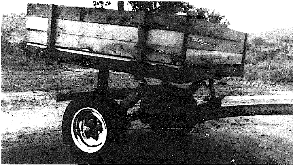
Animal drawn tool carrier converted for use as a cart: Sudan.
