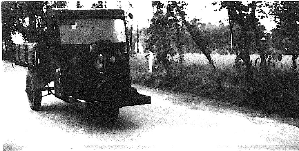
Three-wheeled semi-permanent vehicle in China. The engine can be removed for other duties.
