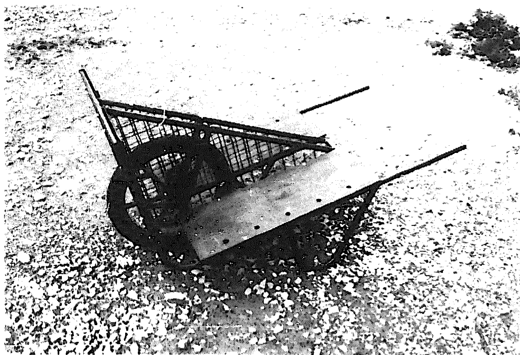
An SFTV made of tubular steel and wood, with pneumatic tyre: U.K.
