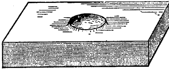
Fig. 87—Showing how the Block is cupped.
