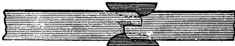
Fig. 95—Welding a Buggy Spring, as done by John Zeck.
