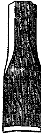
Fig. 48—Improperly Ground Chisel.
