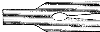
FIG. 181.—SHOWING A FAULTY METHOD OF SPLITTING OUT CROTCHES.
