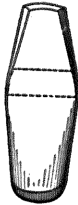
Fig. 68—Showing how the Chisel is Beveled.
