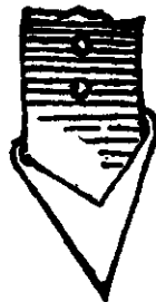
Fig. 389—The Point Adjusted Ready for Welding.
