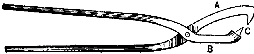
Fig. 42—Iron Tongs for holding Bolt Heads, as made by E. K. Wehry.
