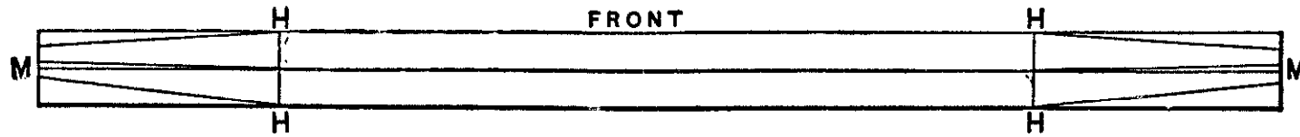
Fig. 152—Showing the Method of Marking for the Gather and Trimming to Fit the Thimble.
