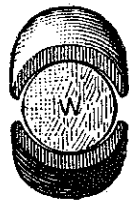
FIG. 142.—SHAPE OF TONG JAWS FOR ROUND WORK.
