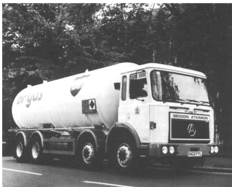
Figure 20.2 LPG road tanker. (Courtesy of BP Oil Ltd)
