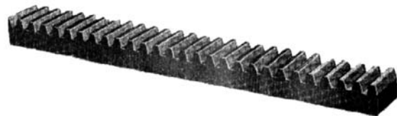
Figure 39.3 Rack or straight-line gear
