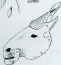
Fig. 8. The mane is then bent forward. The ears are curved around and fixed with rivets.
