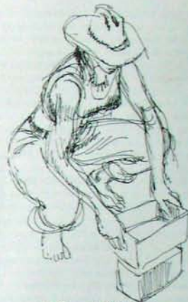
4. Lift mould off the brick
