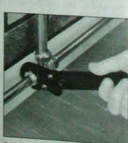
A ratcheting flare nut wrench is ideal for use in tight corners. (Photograph courtesy Stanley Tools)
