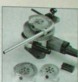
A hired power bender will make light work of bending large-diameter tubes. (Photograph courtesy Ridge Tools)
