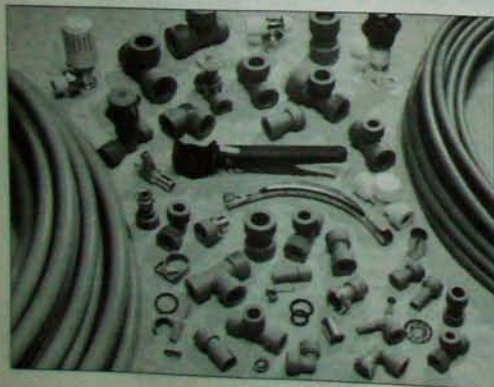
The Hep20 system consists of polybutylene pipe, sized from 10 to 28mm, and a full range of pipe fittings. These include bends, tees, reducers, stopvalves, service valves, etc. Purpose-designed pipe cutters ensure a clean, square cut ready for insertion into the fitting. The system provides everything needed to install a domestic supply network.
