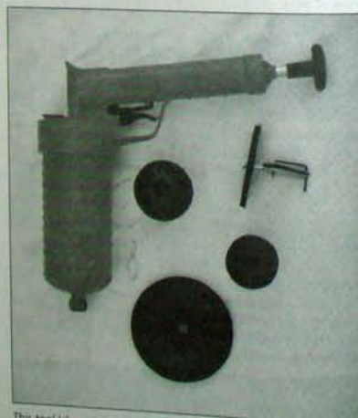
This tool 'shoots' a jet of air into a blocked pipe to break up and force away the blockage.
