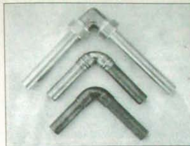
Brass compression, solder-joined and end-feed 90 degree elbows, showing the relative sizes. The bulky compression joint is best used where it will not be seen.
