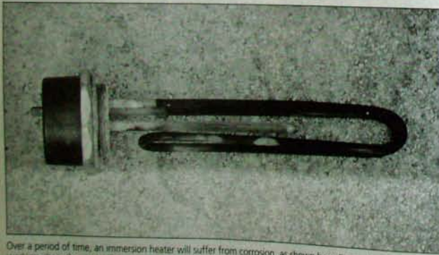
Over a period of time, an immersion heater will suffer from corrosion, as shown here. Eventually, it will stop working altogether and will need replacing. This particular example has short heating elements and is designed for fitting horizontally into the cylinder. Sometimes, two such elements are fitted – one near the top, and one near the bottom – allowing part or all of the cylinder to be heated depending on hot water needs.
