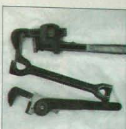
Stilsons, bath/basin spanner and ratcheting wrench. All may be needed when dealing with compression fittings.
