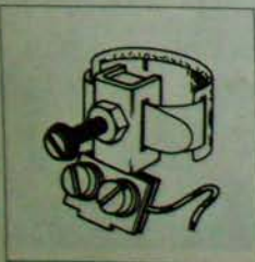
Standard earth pipe clamp (which should be clearly labelled: 'Safety electrical connection – do not remove').
