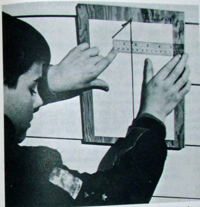
FIGURE 10.12 Homemade instrument being used to determine the declination of a wall.
