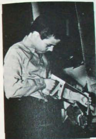
FIGURE 19.4 Making the gnomon for the dial shown in Figure 19.3.
