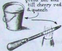
polish sheen on bit end & over blue gas flame draw to bronze color & quench
