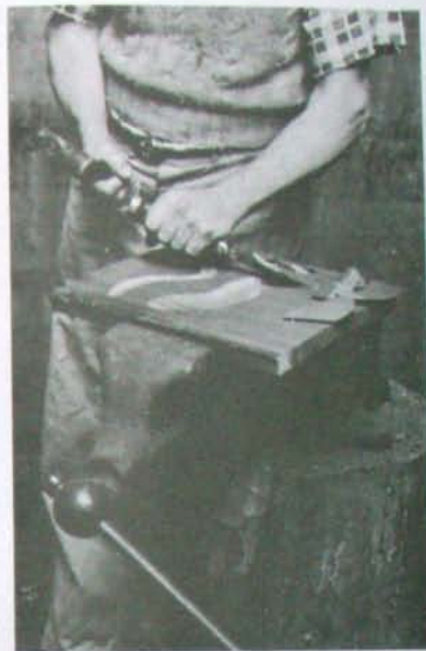
Testing cone design of gouge, cutting an S-curve through splintery, soft, redwood board. The bevel edge is on the outside. The slant of the edge is an original design feature described in Chapter 12.
