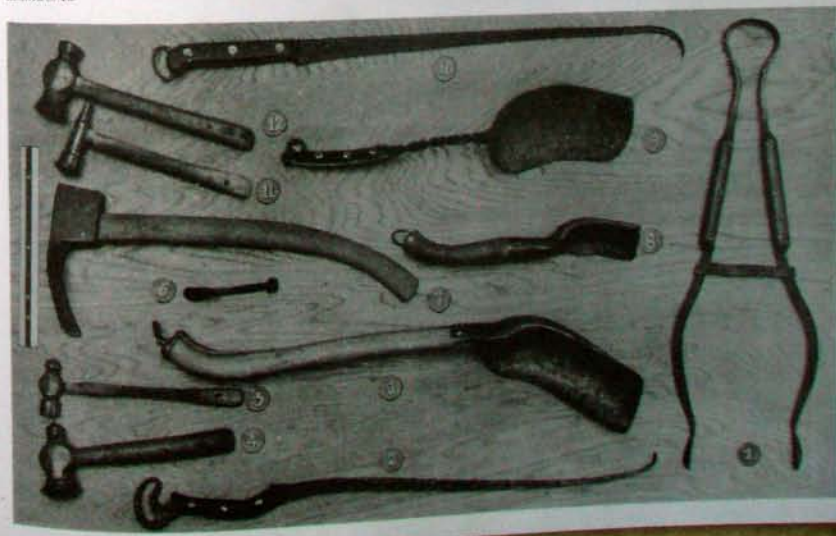
Modern and traditional blacksmith tools and scrap-steel stock: 1 small anvil (hardened face) made from a section of heavy-gauge railroad rail / 2, 3 self-locking pliers (modern vise-grip) / 4 hand-held die-set to form small, round woodcarving gouge blade / 5 standard large cylindrical ground bottom swage, used as stock to make # 6 / 6 special wide-curved cone-shaped blade for a large woodcarving gouge / 7 various sizes of high-carbon-steel rods to make one-point stonecarving tools / 8 hexagon die punch to shape hexagon holes in making box wrenches / 9 hand-held die-set to form keepers for door latches / 10 part of car bumper, which, when clamped in vise, acts as a forming block over which curves are shaped for blades of gouges, shovels, etc. / 11 salvaged spherical section of a ball-joint housing to act as forming block to shape curves / 12 universal hold-down tool / 13 section of a high-carbon bed frame that was used as stock for wood gouge (# 6) / 14 jig, clamped in vise, serves to uncoil heated coil springs into straight rods / 15 single winding of a coil spring / 16, 17 salvaged coil springs from which to make high-carbon, straight steel rod, used as stock for forging small artifacts / 18, 19, 20 keeper blank, forged into final shape / 21 bottom swage made to fit anvil (# 1).
