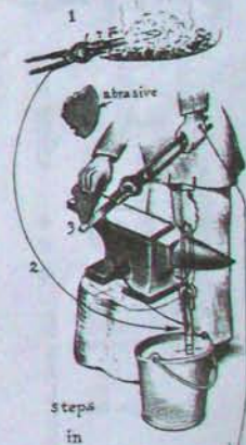
Tempering a cold chisel
