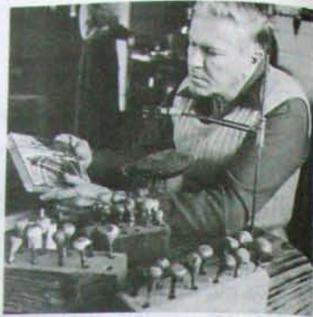
Engraving burins shown on page 276 cut designs on blocks of end-grain pearwood.
