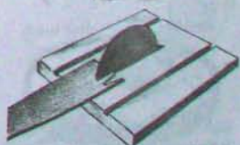
cut teeth on abrasive wheel before or after bending
