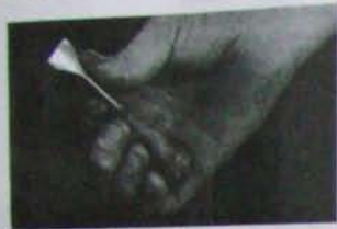
The small woodcarving gouge is manipulated in the same way as the engraver's burin. The flat upright slides along thumb during each stroke of the tool.
