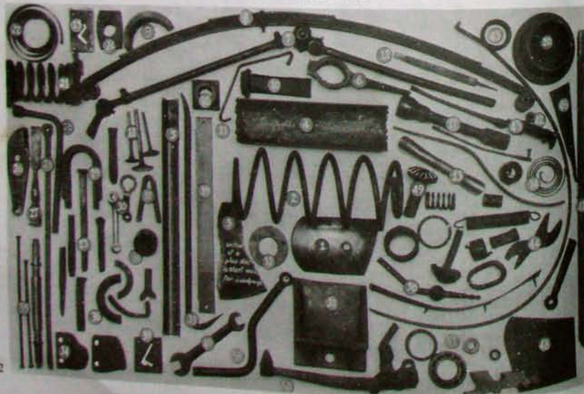
Samples of scrap steel for the modern blacksmith: 1 section of a car bumper / 2, 21 coil spring of a car / 3 section of a plow disc cut with welding torch / 4 half a 4-inch-diameter cast-iron plumbing pipe / 5 angle iron from bed frame / 6 section of a broken pick axe / 7 parts of a steering-gear rod / 8 set of car leaf springs / 9 half of a large ball-bearing race / 10 old wood-splitting wedge / 11 bent 1-x-5/16-inch bar / 12 old flat file / 13 section of a car bumper / 14, 22 old phonograph spring / 15 farm machinery spool / 16 large bolt nut / 17 hub socket wrench / 18 motor valves / 19 industrial hacksaw blade / 20 cast-iron valve-box lid / 23 3/4-inch round bar / 24 large tie-bolt washer / 25, 29 die parts / 26 half of compound shear / 27 old carpenter's flat chisel / 28 hub socket wrench / 29 double maquet / 30 lever linkage / 31 cast-iron bridge shoe / 32 ball-bearing thrust washer / 33 broken crowbar / 34 farm machine cutter blades / 35 engine pushrod / 37 old Ford car maquet / 38 thrust block / 40, 44 old wrench / 42 collar / 43 screwdriver blank / 45 hay-rake tine / 46 scrap-steel-plate remnant / 47 1-x-1-inch high-carbon-steel bar from a harvester's drive shaft / 48 part of a carpenter's hand saw / 49 shaft end and bevel gear / 50 part of a car stick shift, and lawnmower blade / 51 ball bearings / 52 antique car spring / 53 car linkage bar.
