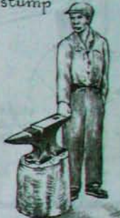
correct height of anvil on stump
