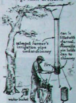
salvaged part of a bulldozer used as anvil small tools easily forged in above setup
