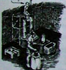
Fuel: teakwood charcoal anvil: broken shaft of sugar mill crusher, set in wood stump Forge: basin. air ducts in clay quenching tub: hollowed out log shop: bambu structure & clay floor
