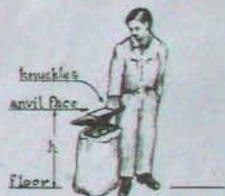
correct height of anvil face from floor level
