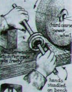
grinding outer bearing race to fit template
