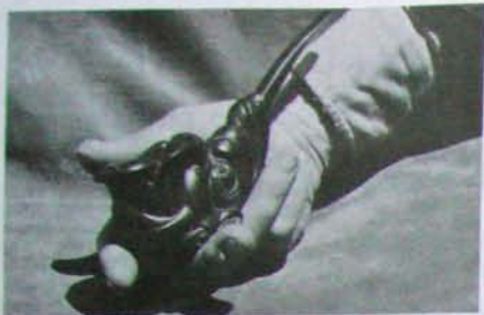
Engraver style wood-carving gouge was used to carve this pipe in mantanital burl.
