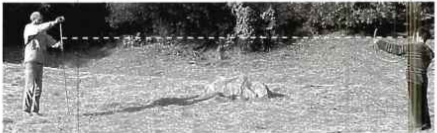
Checking levels with a water transit. Person at right adjusts tubing height until her eye and the near and far water levels are exactly in line (don't drink coffee before doing this!) while person at left moves his finger up and down tape measure until his finger is exactly in line as well. Reading on tape measure minus distance from her eyes to ground is height difference between locations.
