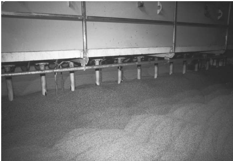
Figure 4.4 A germination “box.” Photograph courtesy of Pauls Malt.
