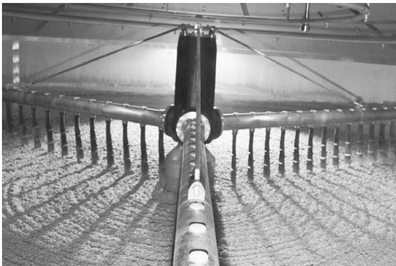
Figure 6.5 The “gear” inside a lauter tun. Courtesy of Briggs of Burton.
