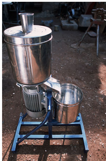
Figure 2: Peanut grinding machine. Example of equipment produced in the Practical Action light engineering workshop. ©Practical Action
