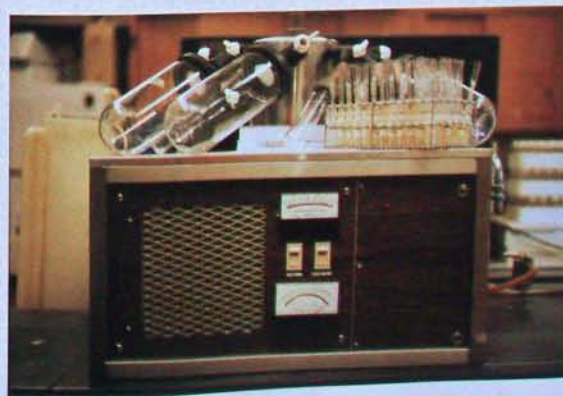
FIG. 11-6 Lyophilization, or freeze-drying, is used to preserve microbial cultures. The instrument used for this process uses a high vacuum and low temperature so that water sublimates (goes from the solid frozen state directly to a gas). This removes water from the specimen without disrupting cellular structures, allowing viability to be maintained.
