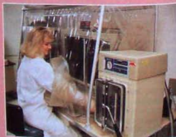
An anaerobic glove box like this may be used to culture anaerobes.
