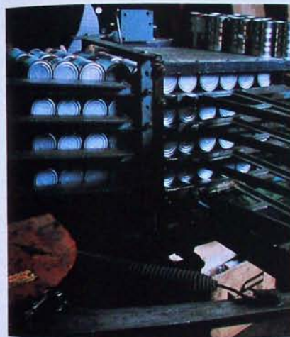
FIG. 11-4 Canning is widely used to preserve foods and keep them free of pathogenic microorganisms. Canning involves heat killing of microorganisms and hermetic sealing under anaerobic conditions to prevent recontamination and spoilage.
