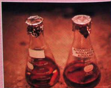
Photograph showing sterility check with special heat-sensitive tape. Left flask is before sterilization and right flask is after autoclaving. The heat sterilization causes the letters on the tape to appear, indicating that the media has been autoclaved.
