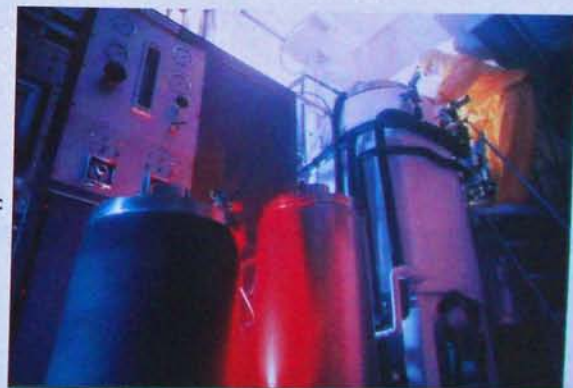
FIG. 1-11 conf'd C, Some vaccines are produced by growing recombinant vaccine strains in fermentors; the fermentor in this photograph is used to produce hepatitis B vaccine employing a recombinant strain of Escherichia coli containing the viral genes.
