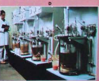
Microorganisms are grown in fermentors to produce pharmaceuticals. Small-scale fermentors are used in the research and development phase of pharmaceutical development.
