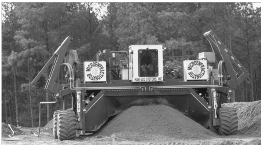
Figure 8. Photograph of field-scale soil mixer. Photo courtesy of H&H Eco Systems, Inc. (North Bonneville, WA).
