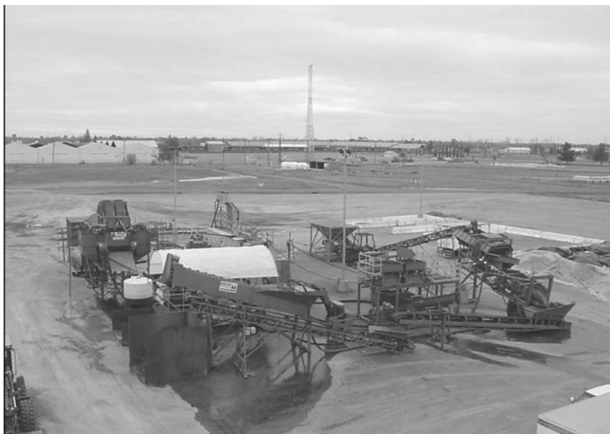
Figure 11. Photograph of soil washing equipment used for physical and chemical treatment of contaminated soils. Photo courtesy of Brice Environmental Services Corporation (Fairbanks, AK).
