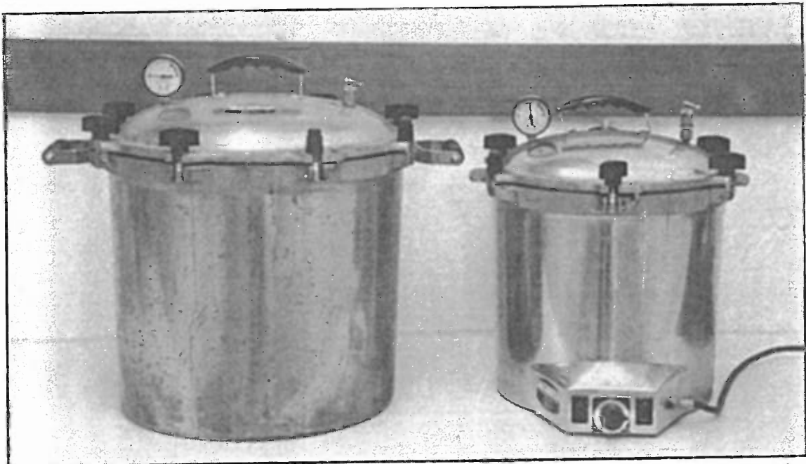
Figure 104. Pressure cookers useful for sterilizing agar and grain media. Note the smaller unit has a built-in heat source. The larger pressure cooker is placed on a stove-top or propane burner. Pressure is regulated by adjusting the heat source.
