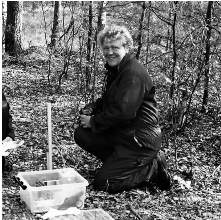
Fig. 14.2. Sampling a gas monitoring well at the Trollberget site in Southern Finland using a portable gas analyzer. The analyzer has an air pump and sensors for measurement of \text{O}_2 , \text{CO}_2 , and \text{CH}_4 . Two gas monitoring wells reaching different depths are installed next to each other.
