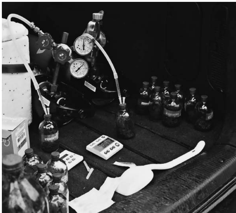
Fig. 14.1. Preparation of anaerobic microcosms in the field. The head space of 120 serum bottles containing soil are flushed with nitrogen gas in the trunk of a car.
