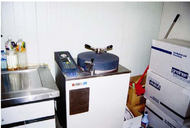
Figure 12. Put the jars in the autoclave and sterilize them at 121 °C for 45 minutes.
