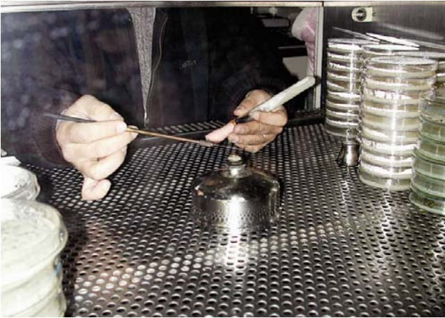
Figure 16. Sterilizing transfer tools and the mouth of test tube by alcohol lamp.
