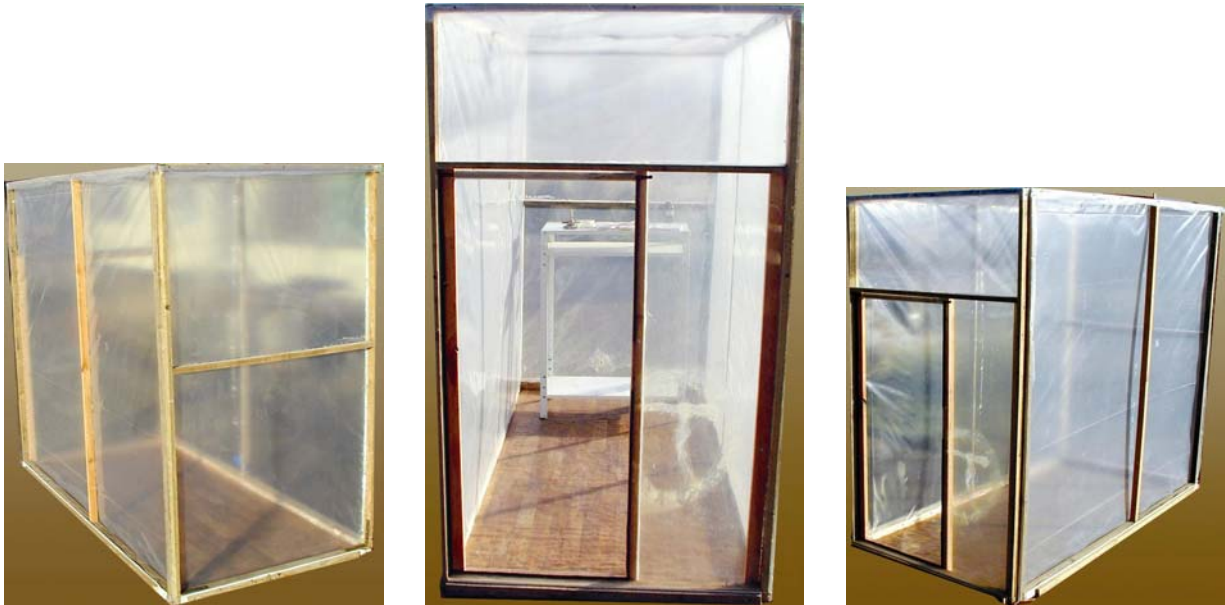
Figure 2, 3, 4. End frames of clean room
