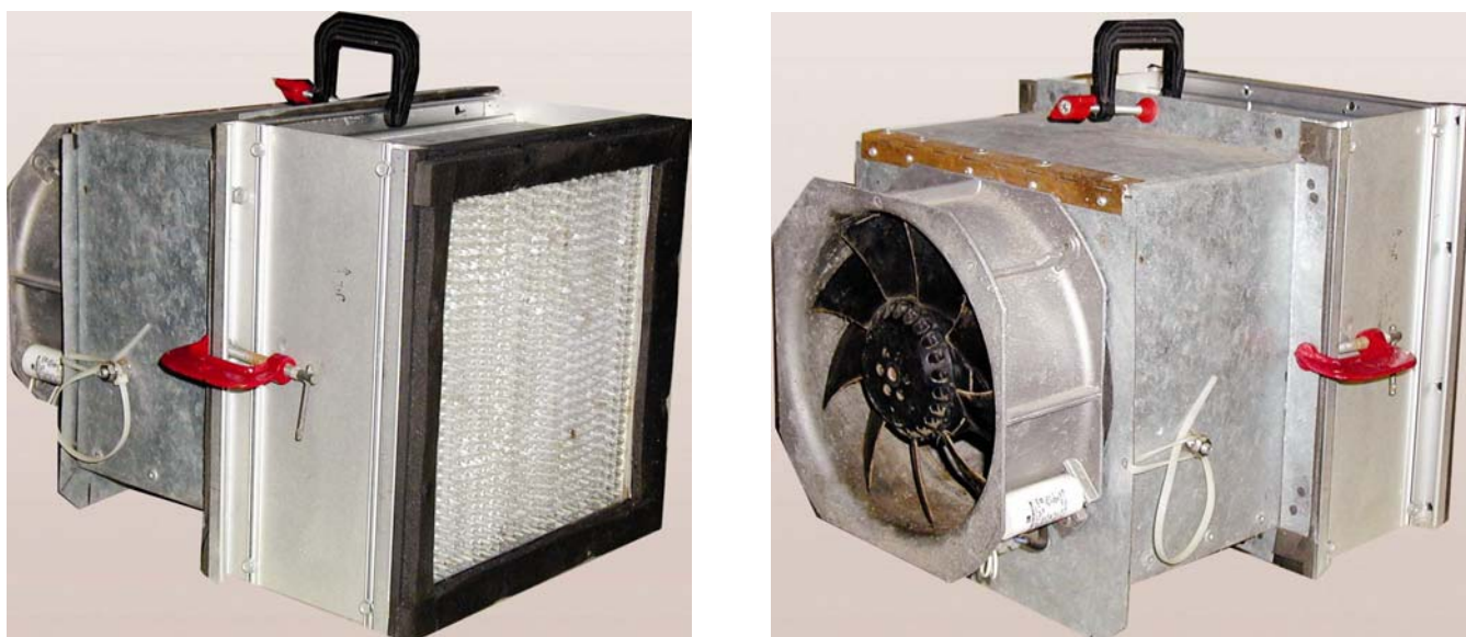
Figure 6, 7. Simply made HEPA filter
