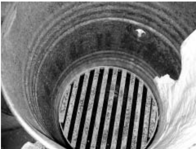
Figure 13. Inside the drum sterilizer
