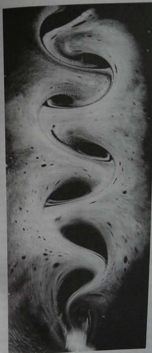
Water Disturbance Pattern. A thin brush has been drawn in a straight line through a shallow tray of glycerine treated water, whose surface has been dusted with powder. (Schwenk method, photo by A. J. Wilkes).
