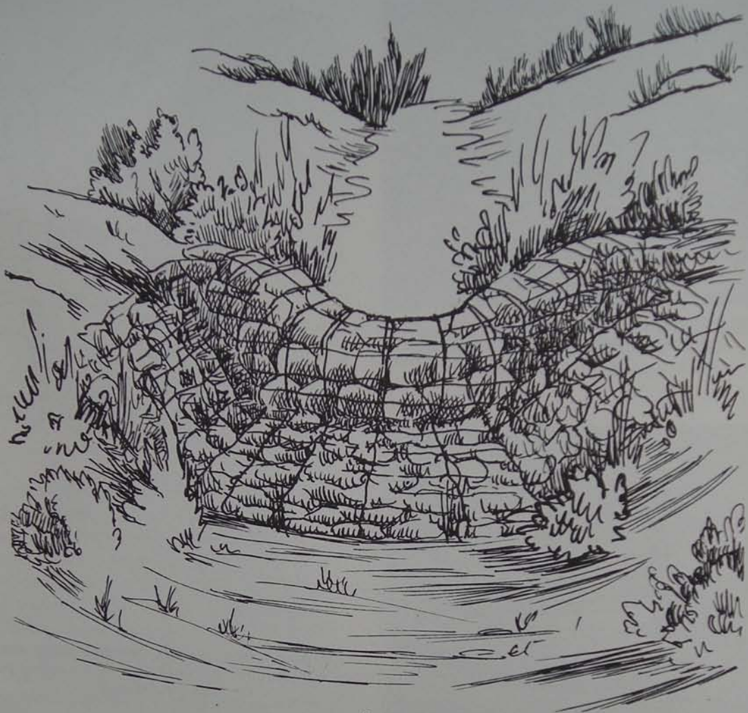
Fig. 3.23. A gabion is a wire-wrapped stone check dam. A wire-wrapped downstream apron prevents erosion at the base of the check dam and dam failure.
