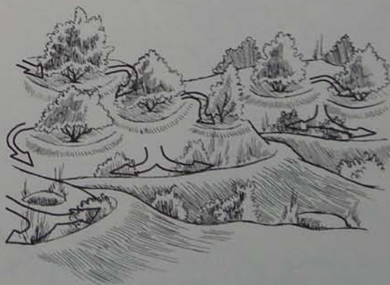
Fig. 3.4. A series of boomerang and contour berms on a sloping landscape. Arrows denote water flow spread and infiltrated by the earthworks.
