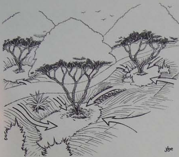
Fig. 3.9. A series of infiltration basins intercepting and infiltrating rainfall and runoff from adjoining street and footpath. Designed right, these basins can act as the sole irrigation system for the associated vegetation, while doubling as a flood control system.
