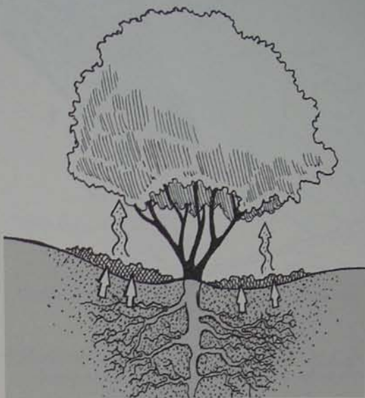
Fig. 3.14B. The basin mulched for improved infiltration and retention of water into the soil
