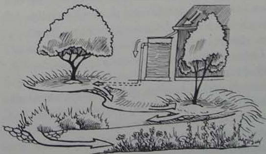
Fig. 1.17. Cistern overflow water directed to, filling, and then overflowing one earthwork to fill another and another
