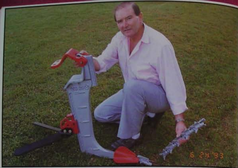
Plate 59 Allan Yeomans shows three of his new patents. Rigid, simple shear pin system uses inexpensive round steel bar. "Leap Frog" digging points fit behind used ones, as shown, which means no throw away metal. Self locking rear track gives quick tool change. Photo shows weed knives.
