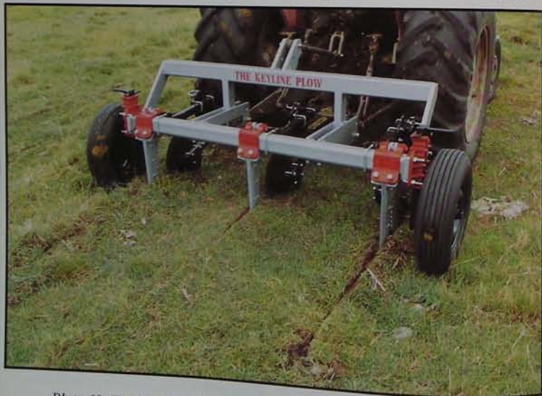
Plate 60 The versatile Yeomans Plow at 300 mm (12 inches) deep aerating and fracturing a hard pan. Over 50 varieties of cultivating points can be fitted and sizes range up to 10 metres (33 feet) wide.
