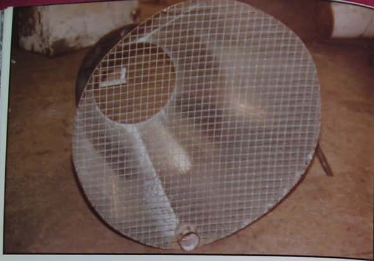
Plate 55 The "cone strainer" for inlet of the Lockpipe System prevents blockages and increases flow rate. Note the 75 mm (3 inch) socket for Flota-filta pipe.
