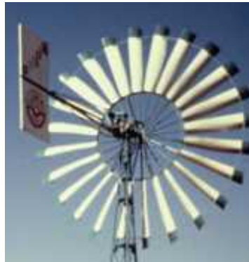
Figure 1: High solidity rotor ©Practical Action
