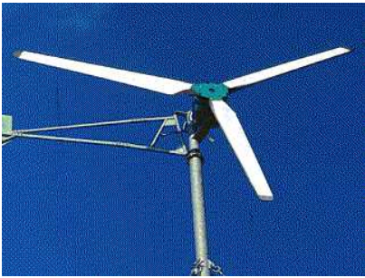
Figure 1: Low solidity rotor ©Practical Action
