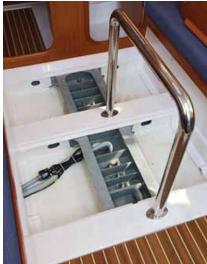
There's plenty of room below for a sail inventory when racing (top). Halyards and sail controls lead aft to the X-35's cabin top (left). The hot-galvanized steel frame inside the hull absorbs the loads from the keel and rig (right).
