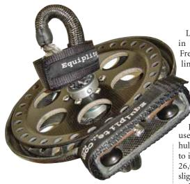
**EQUIPLITE UNITS ARE** used for free-luff sails on boats 30 to 100 feet. All furlers, including the 10 FS (above, for 60 footers and larger) use soft loops, at the drum and swivels, which contributes to its light weight (the 10 FS weighs 3 lbs.)
