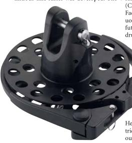
HARKEN CURRENTLY OFFERS a Code Zero continuous-line furler for reaching sails; the smallest unit is designed for boats in the 20- to 30 foot range.
