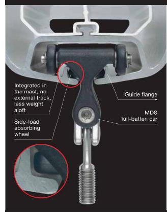
The Seldén MDS system interacts with the mast section making sail handling much simpler. The MDS cars are supported in all directions, running practically friction-free even under heavy side loads created by full-battens.
