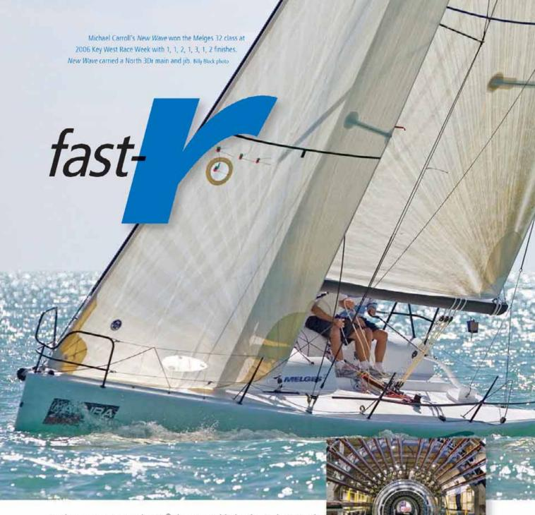
Twelve years ago, North 3DL® thermo-molded sails revolutionized modern sailmaking. Today, another 3D sail revolution begins... it's called <sup>3DY™</sup>. 3Dr sails are manufactured on a highly efficient cylindrical mold that allows North to deliver superior 3D thermo-molded performance — at lower prices and faster delivery times
