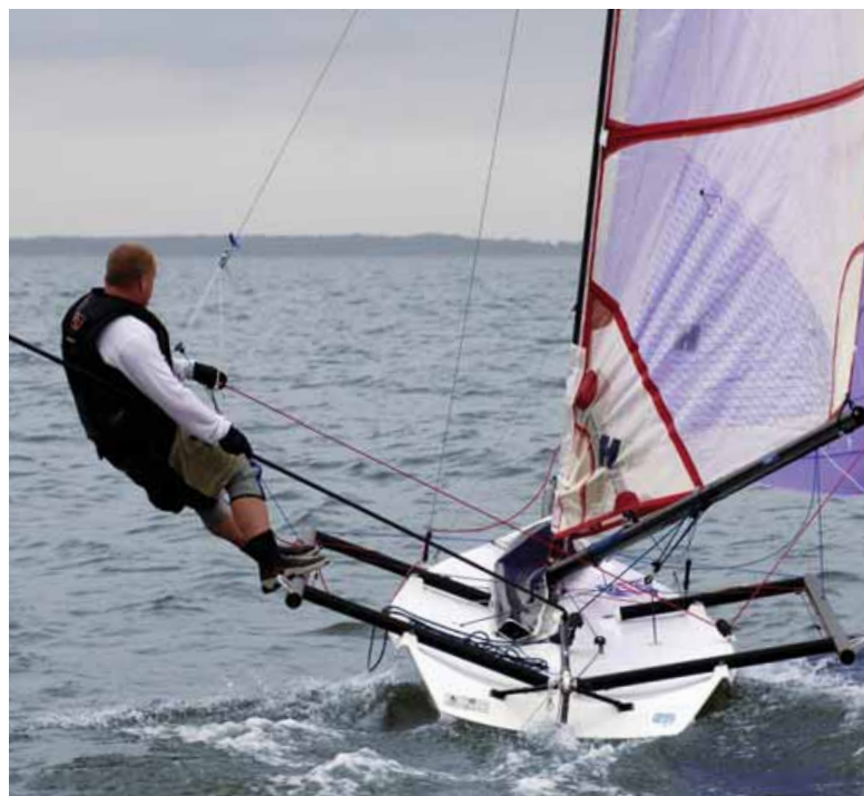
THE MUSTO SKIFF'S large sail area is tamed courtesy of hiking racks. The vang (below) is rigged above the boom.
