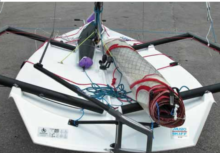
THE SKIFF'S SYSTEMS ARE SIMPLE , allowing for a rig time of 30 minutes after some practice. The port and starboard racks are easy to remove, and they stow inside the boat for transport.
