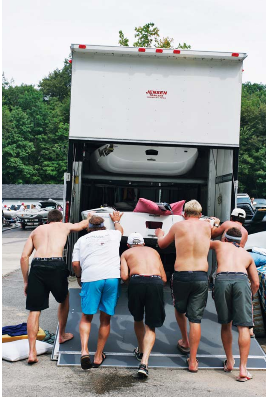
The traveling Avery family, from Lake Okoboji, Iowa, including father, Steve, and sons Fletch and Lance, enlist help loading their enclosed trailer. For this year's Inlands, the trailer brought three C scows, an MC scow, and spars for each. A hydraulic lift positions the C scows three deep.
