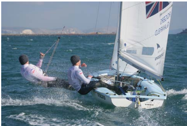
11.2a Boat pointing too high and slipping sideways compared with a boat sailing well.
