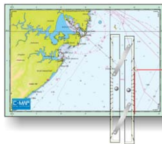
Measuring longitude with a parallel rule
