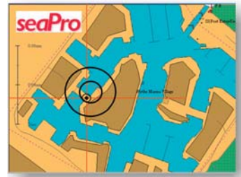
Range rings at 25 metres spacing WAAS GPS errors
