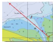
A position line derived from being on a 'transit'
