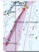
A single position line derived from a linear depth feature
