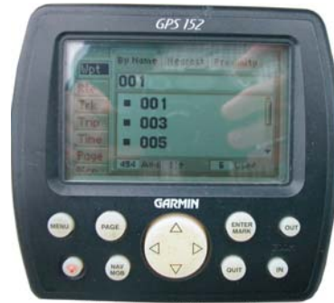
Garmin allows only NMEA waypoints to be transferred, not the whole route. Garmin transfer
