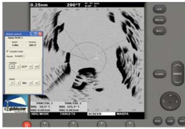
Through entrance, range set at 0.25 mile, heading 290, turning onto a heading of 217(T) to destination.
