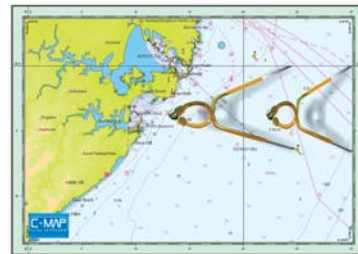
Measuring latitude with dividers
