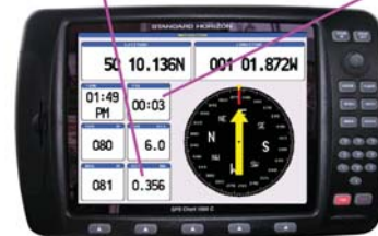
The waypoint is now dead ahead (aligned with the red line, which allows for tide and leeway)
