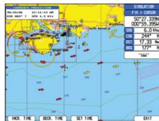
Actual value of tidal flow at the cursor. Using the keys to increment or decrement time in one-hour steps, the change in flow can be investigated. A specific time can also be set.
