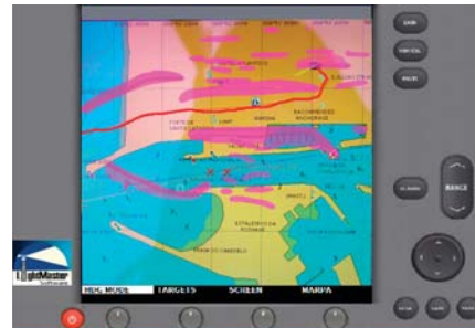
With radar overlay, the chart error is very obvious.
