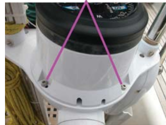
Adjusting compass for 'A' error
