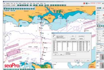
Weather files (grib files) can be down loaded from the internet and the software then allows the winds from these files to be used to calculate the best route to be calculated
