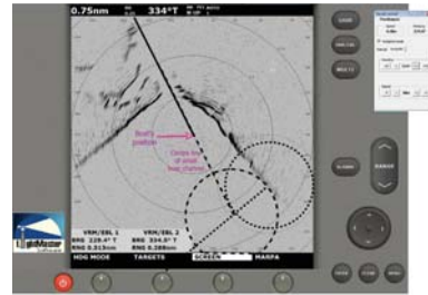
The boat is well along the small boat channel, on its centreline and heading 334T.
