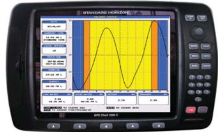
Tidal curve for a designated point
