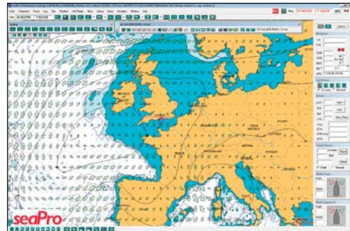
The grid file (weather) can be displayed. If the grid file is for a forecast period of 60 hours, the wind direction and other data if available can be shown for various time intervals.
