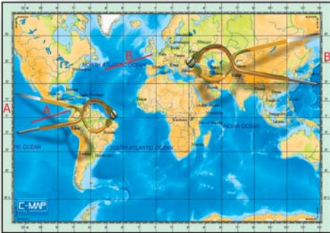
Use latitude scale at same latitude as distance to be measured
