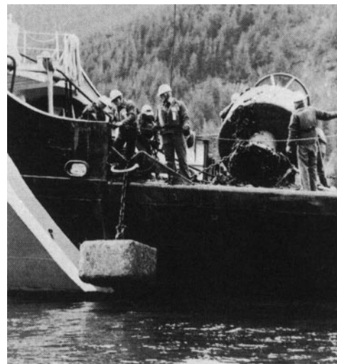
Figure 512. A sinker used to anchor a buoy.
