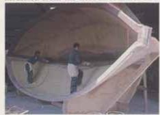
the cold in winter. The insulating quality of Airex virtually eliminates condensation in the hull and makes those storage lockers under the bunks usable again. The ballast is cast lead. And the boottop and sheer stripe are Awlgripped.
