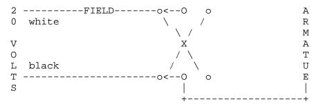
NOTE: no connection at "X"; Include a green-wire frame ground if at all possible
