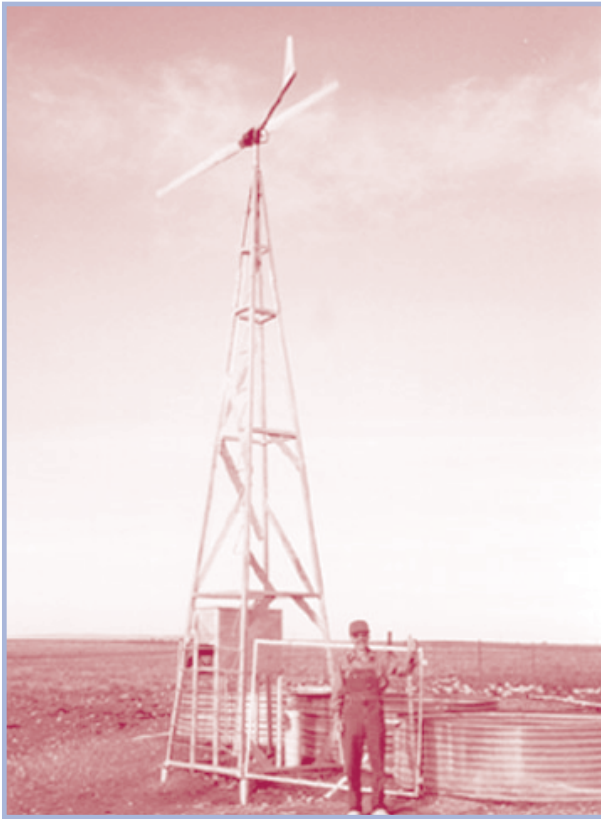
This Texas rancher uses a wind-powered turbine to pump water for his cattle.
