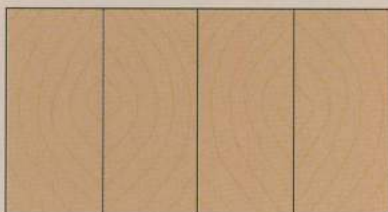
Book-match A repeating pattern where adjoining sheets of veneer appear to radiate from the joint between them, like the pages of a book
