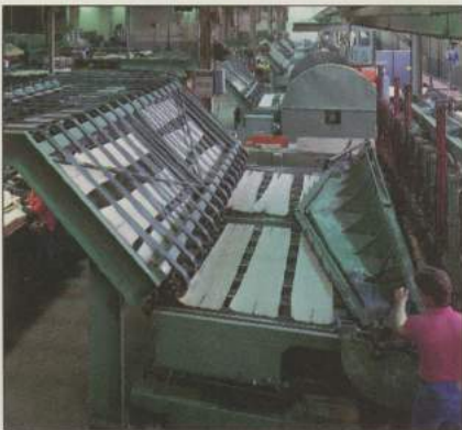
Flat-sliced sheets of veneer move along a conveyor for drying and storage in a veneer factory.
