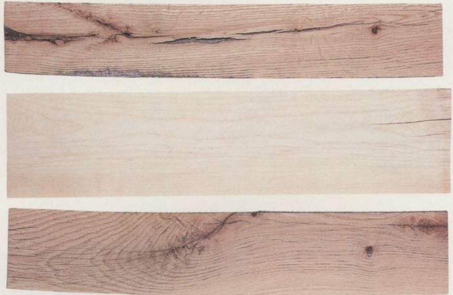
Three pieces of oak with defects: The top board shows splits, the middle piece reveals checks at one end, and the bottom board displays a crook, a loose knot and reaction wood.
