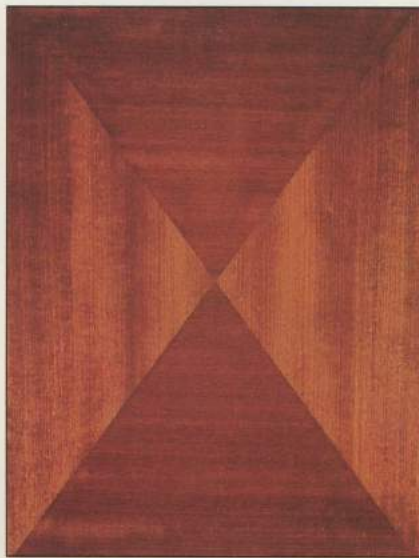
Artfully matching veneers can create eye-catching effects. This tabletop features a center diamond match.
