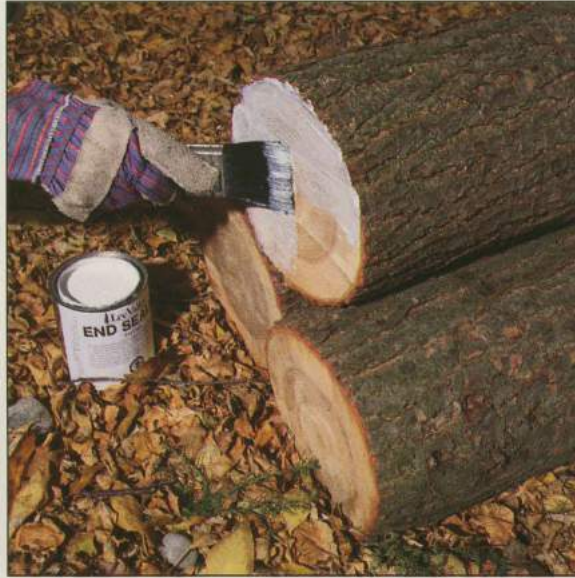
Logs for carving can be stored in a pile one atop the other, provided their ends are not in contact. The ends should be coated with a sealer, however, soon after the logs are bucked to ensure even drying of the wood.
