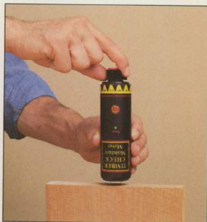
A resistance moisture meter like the one shown above is a cylindrical device with two pins that are pressed into a board. The meter measures electrical resistance, which will vary depending on the amount of water in the wood.
