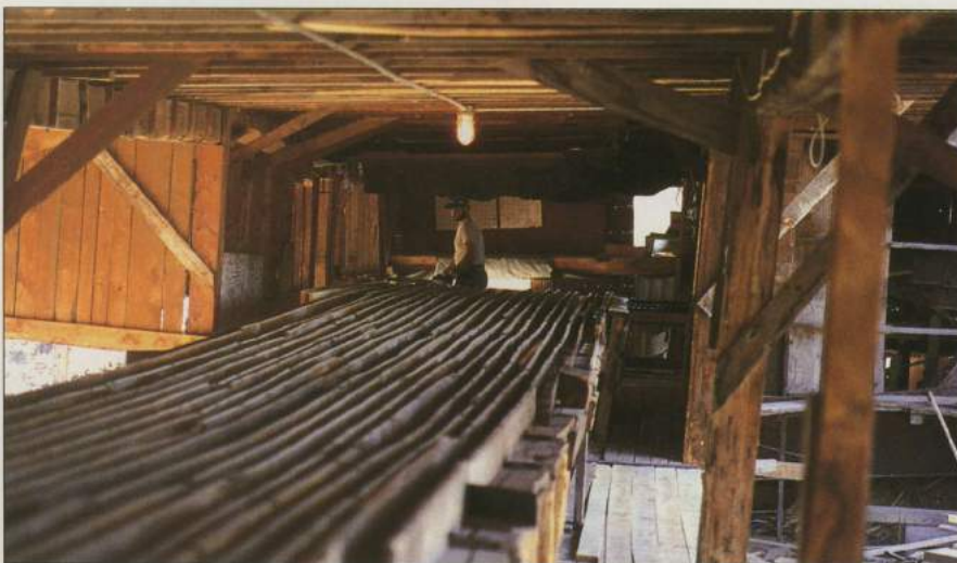
A device known as a “slot machine” sorts freshly sawn boards into the right widths and lengths.
