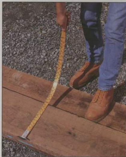
Principal tool of the lumber grader's trade, a lumber ruler measures the width of a board. With a flexible shaft and a hook at one end for flipping stock, the ruler enables a grader to fill an order for wood quickly.
