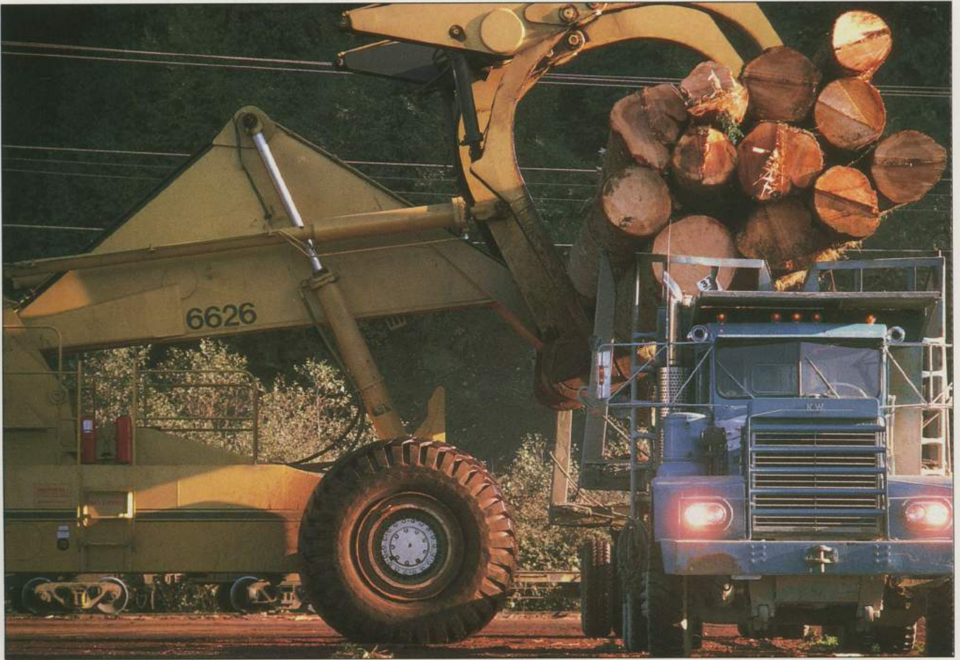
A hydraulic log loader dispenses its contents onto a truck.
