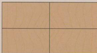
Butt-and-book-match Commonly used with butt, crotch and stump veneers to create an unfolding, circular effect
