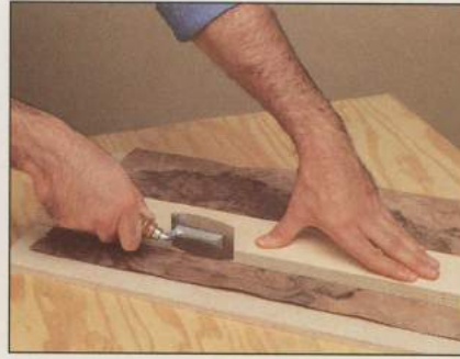
Specifically designed for cutting veneer, a veneer saw is usually used in tandem with a guide block or a straightedge to ensure straight cuts.
