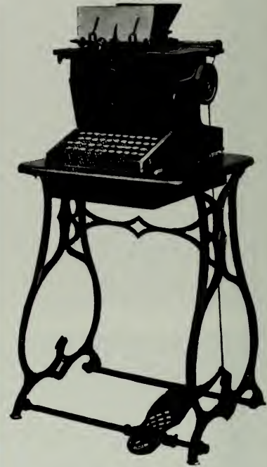
The first typewriter (above) During the late 1860s, the Americans Christopher Sholes, Carlos Glidden and Samuel Soulé developed the first machine to write faster than the hand – the forerunner of the modern typewriter. The first model went on sale in 1874, manufactured by the gunsmiths Remington and Sons.
