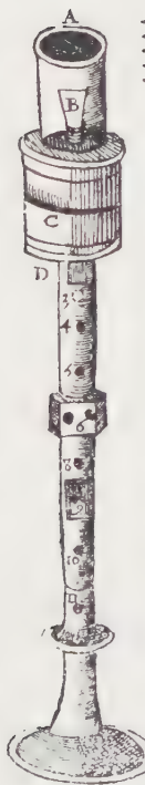
Fig. 9. Diagrams showing the construction of the musette. From Mersenne, Harmonie universelle , 1636. In upper diagram under R, and in lower diagram under N and O, note the four oboe reeds corresponding to the four drone channels concealed in the bourdon cylinder. In lower diagram, note the layettes marked L. The chanter shown is the form in use before Hotteterre's invention of the petit chalumeau .
