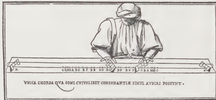
Fig. 5. Monochord for studying consonances; the two stopping bridges permit two tones to be produced simultaneously on a single string. Woodcut from Lodovico Fogliano, Musica theorica , 1529.
