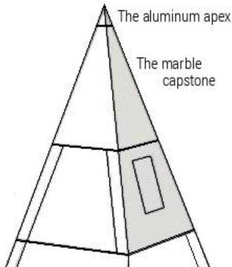
Figure 9. The marble capstone on the top of the pyramidion.
