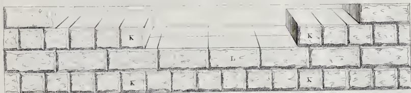
K, courses of the lesser stones. L, courses of the larger stones.
