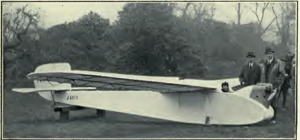
FIG. 6.—The "Wren" 3 h.p. Monoplane, 23 ft. long, span 37 ft., speed 50 m.p.h.
