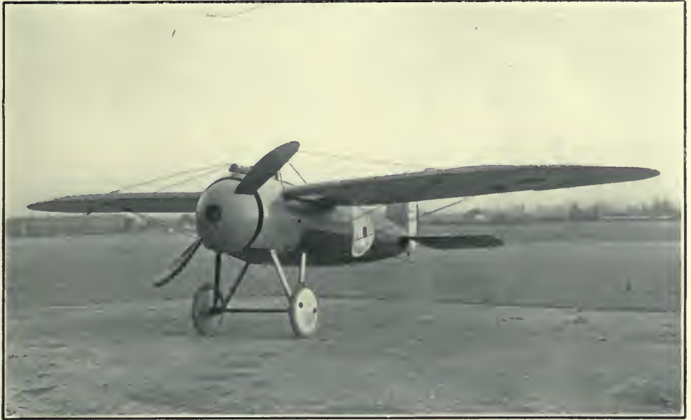
FIG. 1.—A 110 h.p. Bristol Monoplane. Note the cowling over the centre of the tractor screw.
