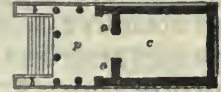
Plan of Roman prostyle temple. Temple of Augustus at Pola, Istria: a, a, ante; c, c, cells; b, b, projecting piers of podium.
