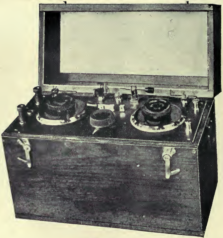
FIG. 5. A portable Receiver, having the Valve arranged inside, out of harm's way.
