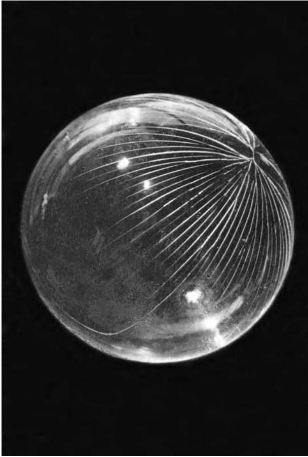
Nasmyth, James and James Hill Carpenter. Glass Globe. Cracked by internal pressure illustrating the cause of bright streaks radiating from Tyoho. The J. Paul Getty Museum, Los Angeles © The J. Paul Getty Museum.
