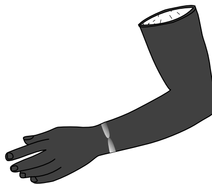
10. Hand joined to arm by flow weld.
