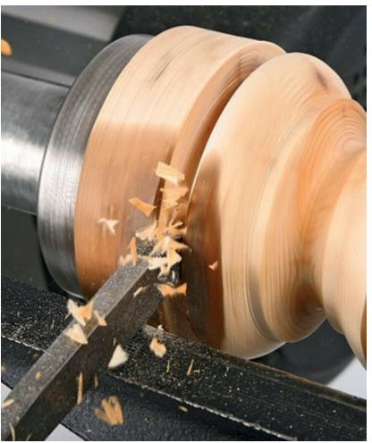
Turned woodwork may be used as part of other wood constructions, but some items can be made entirely on the lathe, such as bowls and tool handles. Turning wood could only be a part of a traditional woodworker's hobbies. Although some craftsmen find some interest in the lathe, they do very little besides turning wood. Lathes seem to have been used nearly since man first mastered the use of tools.
