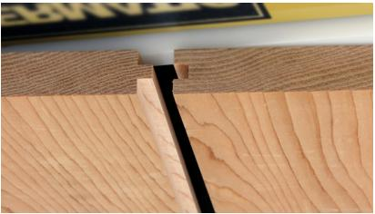
You may easily mount the joint and tie it together with the fasteners when you link two boards close to each other alongside. This joint is far stronger and has more adjacent surface areas, that can be especially useful when you are trying to glue the joint.
