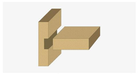
A joint dado consists of a square-grooved boards that fits into another board on one side. Like the tongue-groove joint, this one is also a wood joint that is commonly used for joining plywood for cabinet making.
