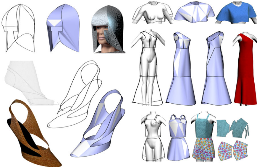
Fig. 14.17 Developable helmet, shoe and garments generated from their 3D boundaries
