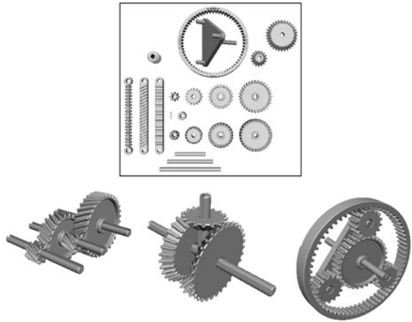
Fig. 10.31 The gears were assembled using transformation strokes in conjunction with standard transformation techniques
