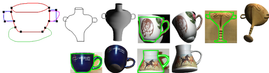
Fig. 6.8 The cup template graph, and sketches of cups and wine glasses shown together with the synthesized 3D models
