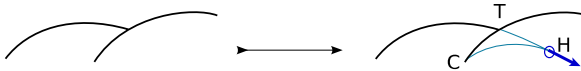
Fig. 12.10 When we have a T -point and a cusp to match it to, we seek the location of a hidden cusp such that the two hidden contour parts joining our points to the hidden cusp have the highest probability
