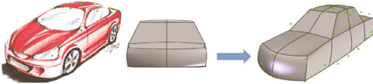
(b) Template alignment. Left: Input sketch with marked fiducial points. Middle: Initial template configuration. Right: Aligned template in relation to fiducial points.
