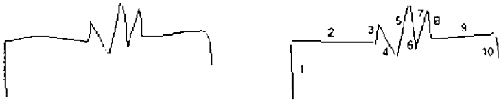
Fig. 5.9 A hand-drawn resistor ( left ) and the segmented ink ( right ). (From [9]; used with permission)
