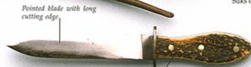
Hilt made of antler riveted to tang of blade
