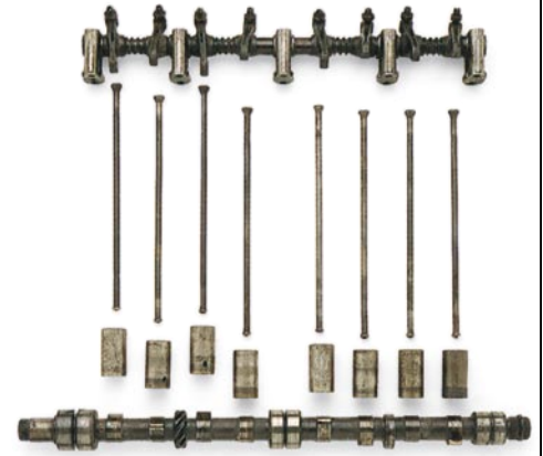
VALVE TRAIN In older engines, the camshaft is at the bottom of the engine near the crank, and the valves are operated through a series of rods called pushrods.
