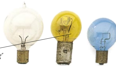
Early double-element "dipping" headlight bulb
