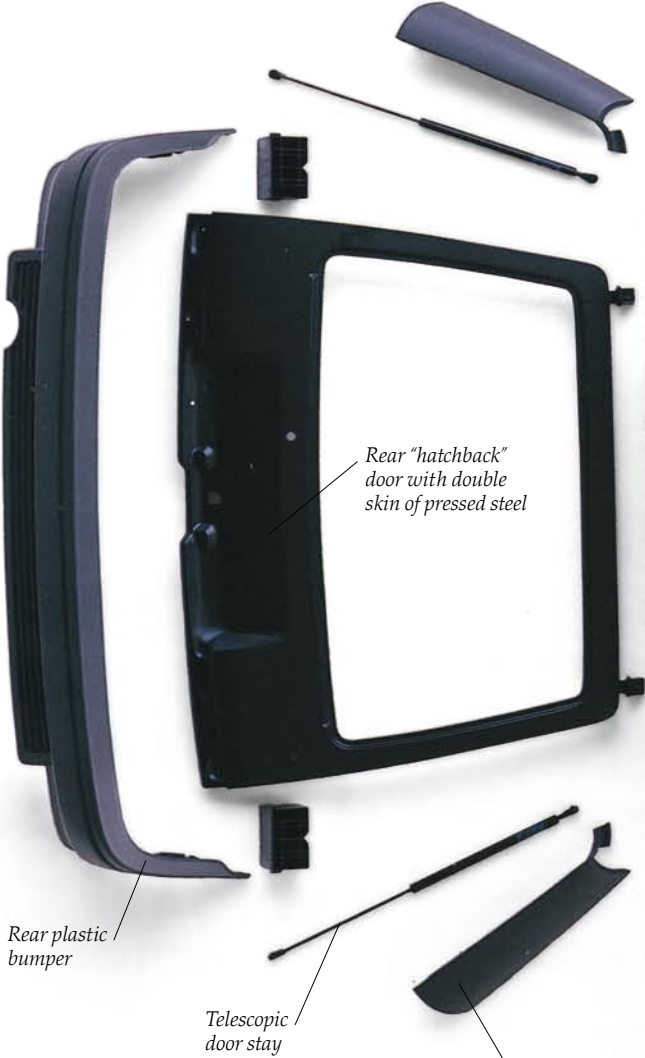
Plastic trim panel to cover electrical wiring access
