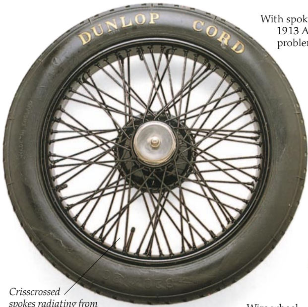
Wire wheel and disc cover
