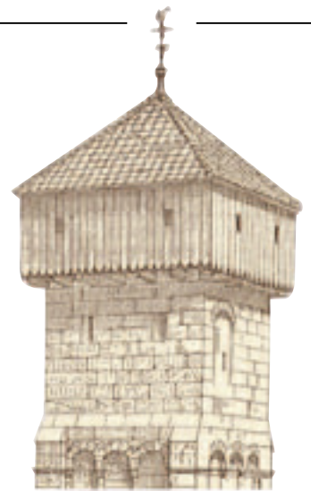
HOARDINGS Removable wooden hoardings were supported on beams pushed into holes below the battlements.
