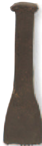
MASON'S CHISEL Chisels were used for cutting and dressing stone, although some stone was soft enough to be cut with a saw. A smithy was needed on site because the tools wore out quickly.
