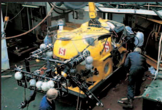
Solo (above) is an ROV used for pipeline surveys and other underwater work in the North Sea oil fields.
