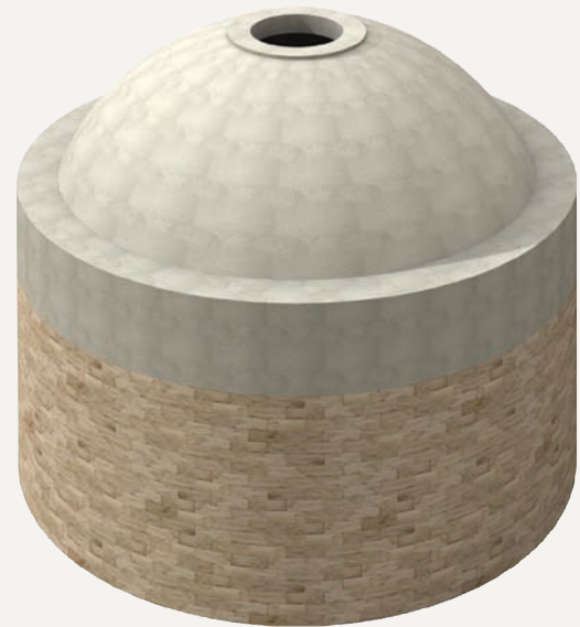
Hemispherical dome with oculus
