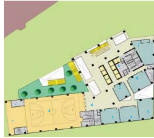
1. stage and backstage area 2. store room 3. multi-purposes hall 4. building line above 5. classroom 6. AHU 7. lecture theatre
