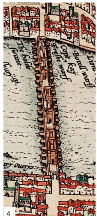
▲ OLD LONDON BRIDGE By the 16th century, this masonry bridge was overpopulated with towering buildings, and the narrow waterways between its piers had become extremely hazardous. The bridge was irrevocably damaged during the fire of 1666.
