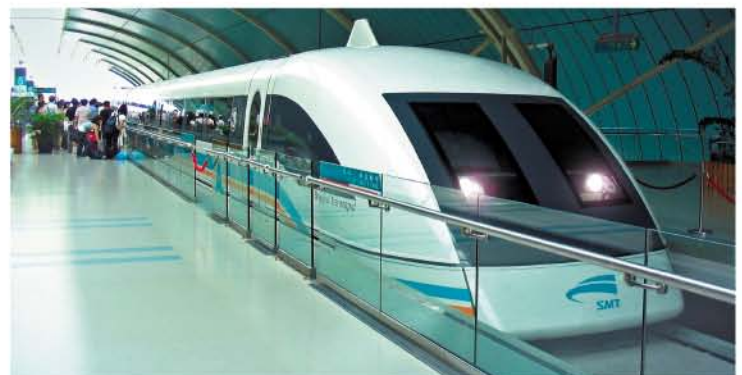
Maglev, China The Maglev, for Magnetic Levitation, is a train that uses magnetic forces to move and is therefore not in contact with the rails when it runs. It has reached a speed of over 500 km/h.
