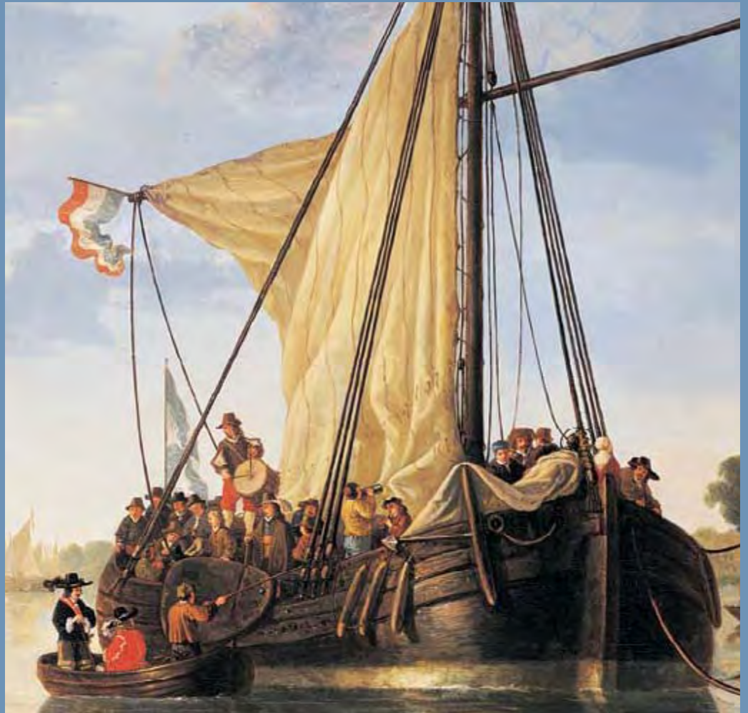
The single-masted pleyt was commonly used as a ferry because it rode high in the water and could negotiate shallow inland waterways. Drawn up along the hull is a sideboard that provided stability under sail.
