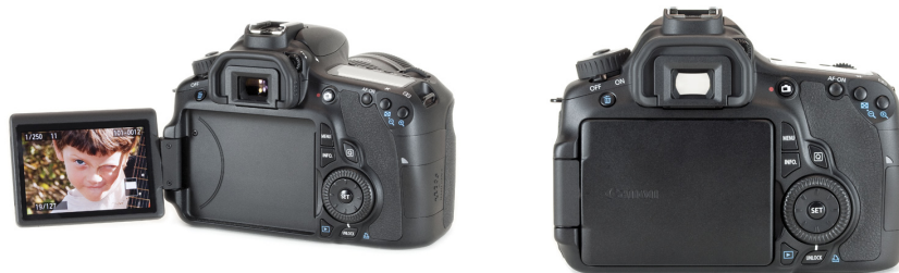
Figure 2-11: Articulated monitors can be positioned very flexibly. You can close them up tight.
