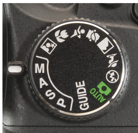
Figure 2-16: Top: The Canon EOS 5D Mark III sports a minimal mode dial. Bottom: The Nikon D3200 has many more shooting modes.
