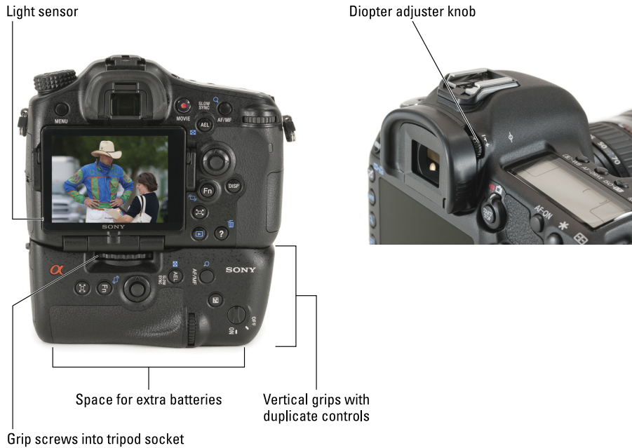
Figure 2-10: This camera is an impressive sight to behold; use its small wheel to adjust the viewfinder to your eyesight.
