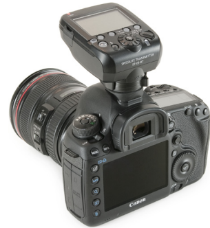
Figure 2-6: This is a dedicated wireless transmitter.
