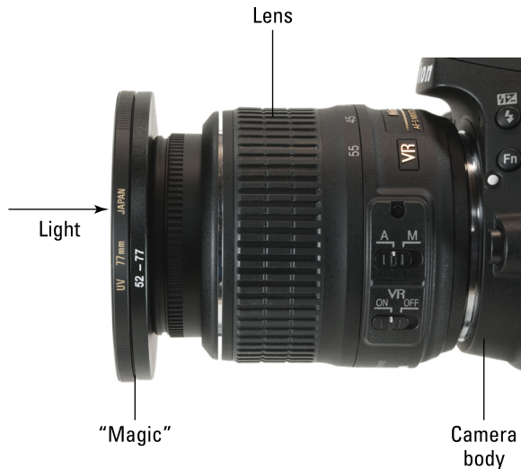
Figure 4-1: Light must pass through the filter for it to work its magic.
