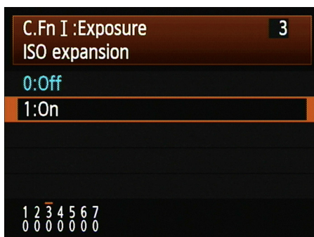
Figure 3-2: Turning on ISO expansion lets you get to the really high ISOs.
