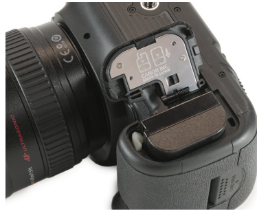
Figure 4-12: A spring pushes up the battery a bit.
