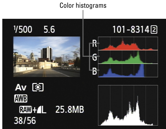
Figure 5-17: In this case, the color histograms are colored to match the channel.
