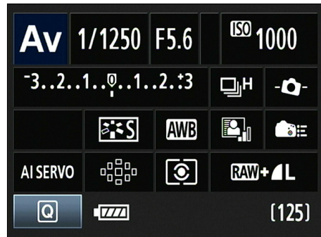
Figure 5-15: The Canon Quick Control screen showing all the important shooting options.
