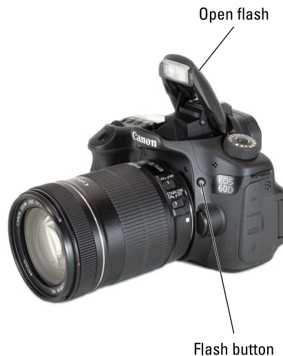
Figure 2-5: Pushing the flash button opens the flash when you aren't in an automatic shooting mode.
