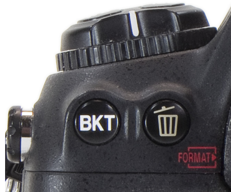
Figure 4-7: This camera has a dedicated Bracket button.
