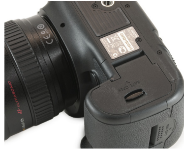
Figure 4-10: Slide the catch to release the door.
