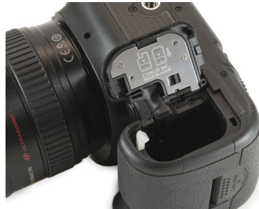
Figure 4-10: Slide the catch to release the door.
