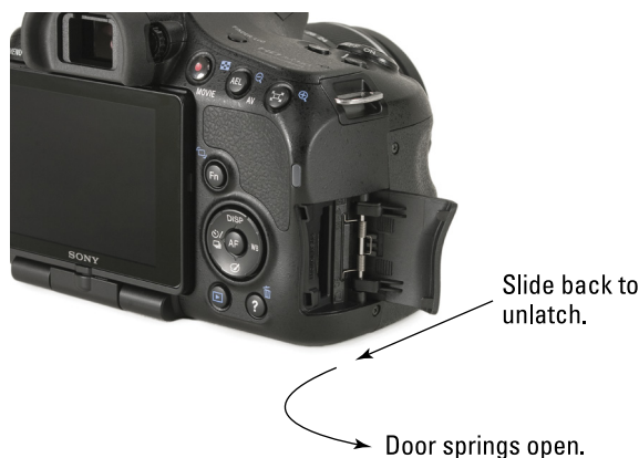
Figure 4-13: This cover slides back and then swings open.
