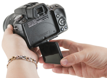
Figure 4-4: An LCD monitor can go from being put away to being pulled from its protective cocoon and flipped around.
