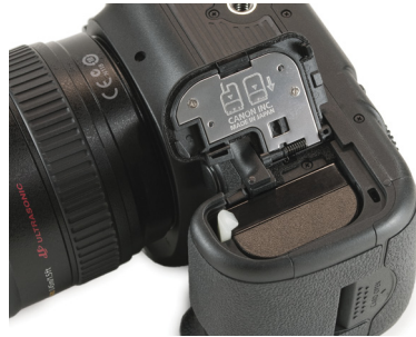
Figure 4-11: Be sure to move the locking lever out of the way as you insert the battery.
